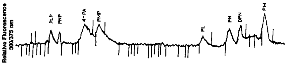
Fig. 1. Representative chromatogram of B 6 vitamers and 4-PA in combined standard solution containing 5 ng of each. The retention times were as follows: 1.0, 1.6, 4.2, 5.4, 14.0, 16.4, 17.3 and 19.4 min for PLP, PNP, 4-PA, PMP, PL, PN, DPN and PM, respectively.
